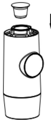
4. Press down and screw down the outlet
