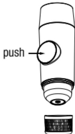
9. Thunder Espresso will automatically stop when finished dispensing. Pressing the button again will stop the machine.
